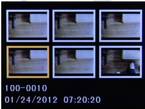
Use the joystick to navigate through the thumbnails. To select a file, press inward on the joystick.
