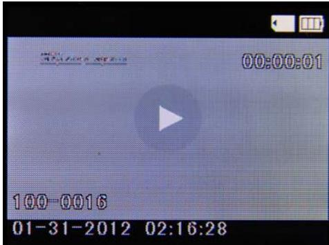
When on playback mode, the bottom left side of the LCD screen will display the file number, date and time. In playback mode, all video, picture and audio files are here and can be played back. The files will start at the most recent file.
