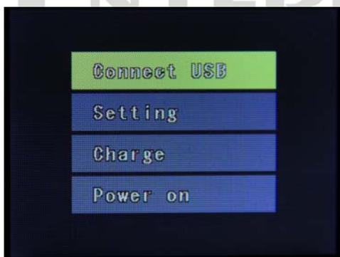
2. Unlatch the “HDMI PC” rubber cover. Take the USB cable and plus the mini USB end into the Wolfcom 3<sup>rd</sup> Eye in the mini USB slot. Plug the USB end of the cable into the AC adapter. Plug the AC adapter into a wall socket. A menu screen will appear. Push the joystick in the down direction until “Charge” is highlighted. Press inward on the joystick and the unit will begin charging. The red LED charging light will turn on.
